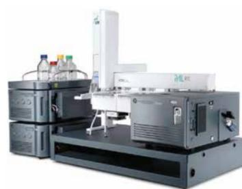
Figure 2: Waters Acquity UPLC M-Class system with HDX technology used for HDX/MS studies
